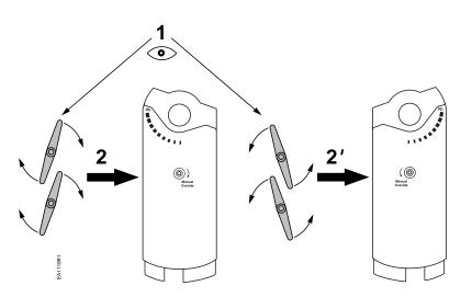
**NOTE:** The actuator can be mounted for clockwise or counterclockwise rotation of the damper shaft. **Figure 2. Actuator Mounting Orientation.**
